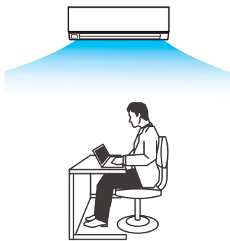
Ideal air flow discharge on cooling mode
