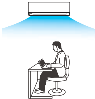
Ideal air flow discharge on cooling mode
