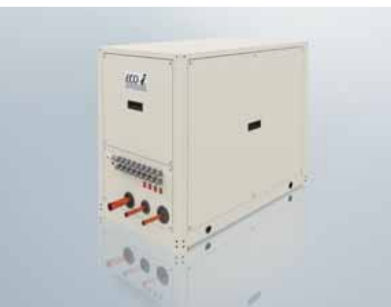
Panasonic offers a purposely engineered solution which allows for a quick and simple installation. The unit contains 5 actuating ball valves, a 30l storage vessel and PLC all housed in an IP54 rated container. Terminals on the front of the unit allow for easy wiring to the alarm terminal, high / low pressure transducers and discharge temperature sensor(s) of the condensing unit(s).
